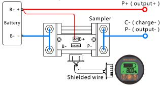
**Attention:** Please connect as shown strictly. The sampler must be connected to the negative circuit, it is forbidden to connect to the positive circuit. If you want to extend the shielded wire, you must use 4 lines of same specification.
